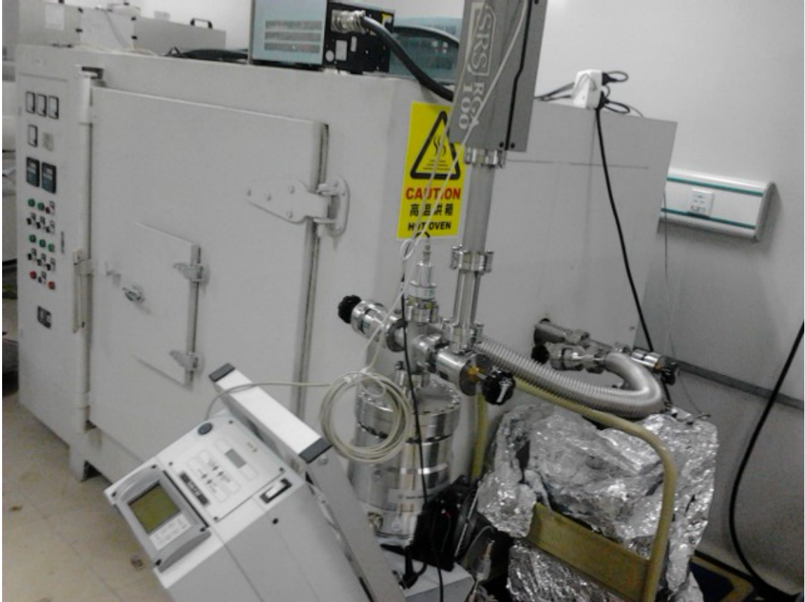
Figure 2.2.3: Vacuum pumps and big oven for baking ion trap and other vacuum components.
